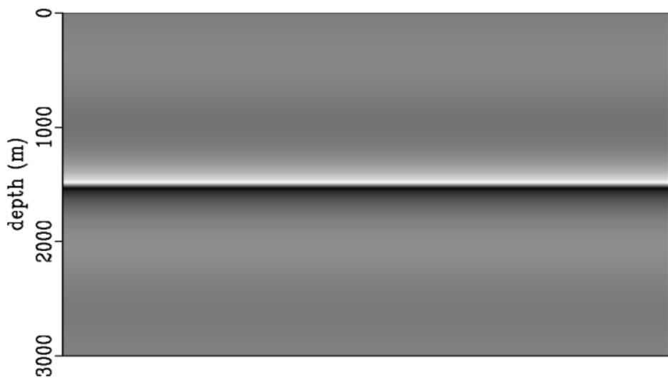
Figure 5: Zoom-in of Figure 4 The new M-OSRP Claerbout III (Stolt extended) migration for 2 way wave propagation. The example with  $c_0/c_1$  velocity. The image both above and beneath the reflector. No “rabbit ears”. Consistent image along the reflector. Light color – image from above. Dark color – image from below. (Qiang Fu and Weglein, 2015)
